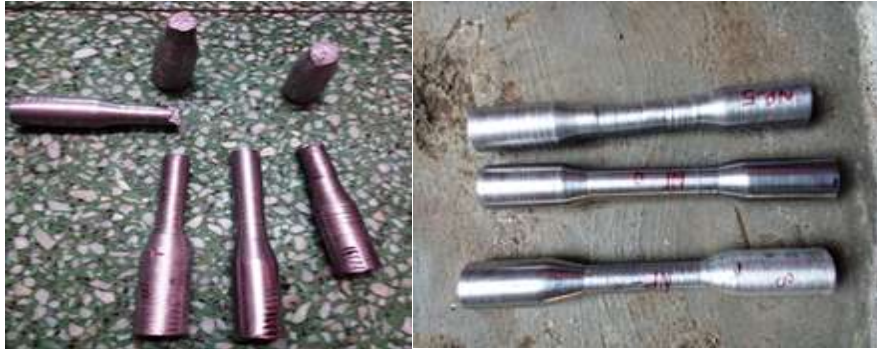
Fig.4 Specimen for tensile testing; before and after fracture
